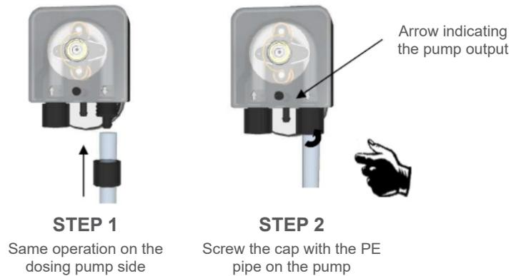
**Mounting procedure for flexible suction pipe:**
