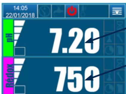
Press on pH to prime acid pump, press on Redox to prime Chlorine pump or chlorinator
